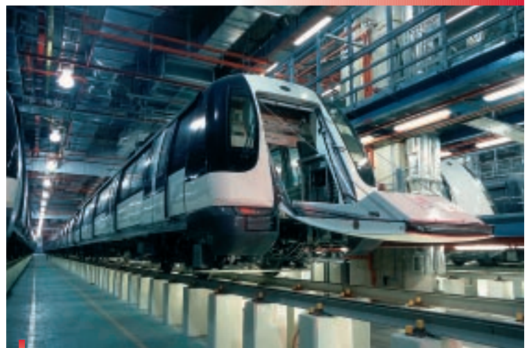
Front-end emergency exit
