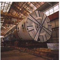
Tunnel boring machine for the second line
